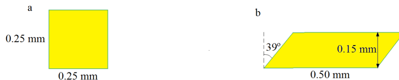
Fig. 8. Change in Lagrange's mesh during asymmetric three-roll rolling process: a – initial mesh; b – mesh after the second rolling pass
